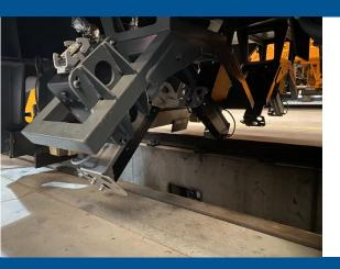
**Side Rail Inspection System** is a machine vision system composed by 4 boxes contact-less, installed on the bogie of the vehicle, two boxes for each rail.
