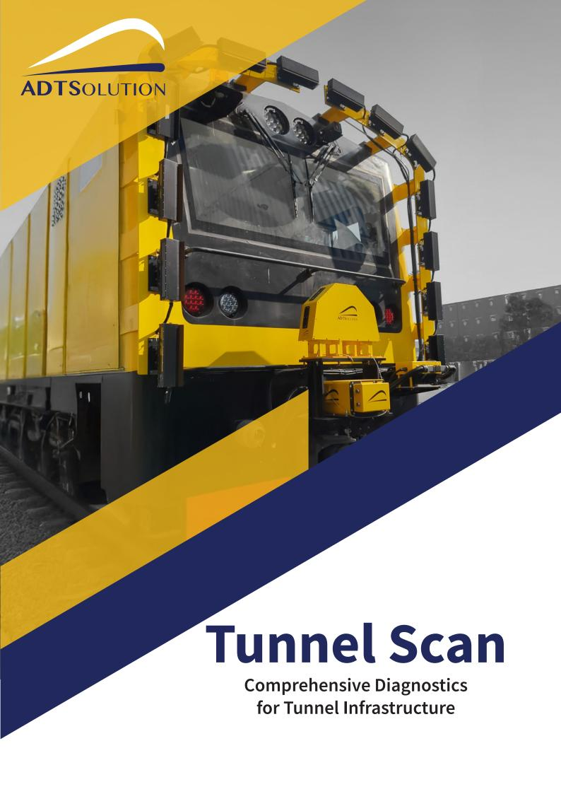
The Tunnel Scan (TS) System takes railway tunnel inspection to a new level of information quality and completeness, providing high-resolution imaging and 3D profiling in a single pass.
