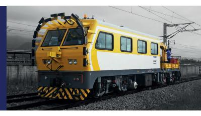
The TS system scans tunnel walls with 1 mm resolution, both longitudinally and transversally, at speeds up to 60 km/h. The entire structure is captured in one sweep, ensuring efficient and complete data acquisition.
