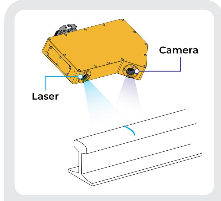
The laser projects a line onto the rail, while the camera captures the profile along the entire track.
