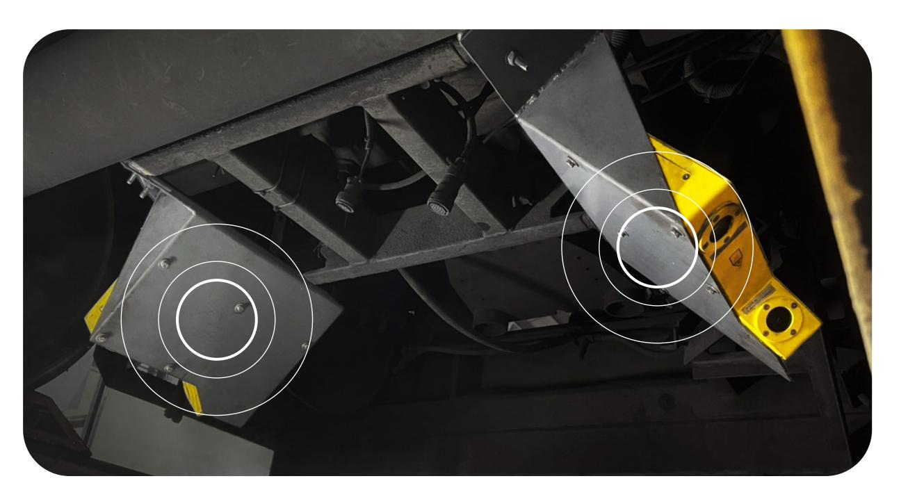
The Rail Profile Measurement System is an optical diagnostic solution for high-precision, non-contact rail profile detection.
